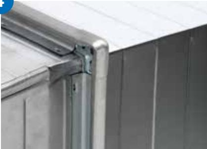
If the duct system is mounted near an evacuation route or pedestrian bridge, there is a risk of someone getting hurt against these corners. To eliminate this risk, or for a neater corner, a corner protection (LS-5) can be fitted.
