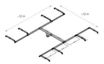
All the duct systems were installed in the ceiling in accordance as per this diagram. The system can be regarded as a typical subsystem in a ventilation system for offices or hotels.
