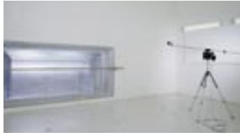
In the reverberation room (4) the sound pressure is measured using a Brüel & Kjær microphone (5), mounted on a rotating boom. The reverberation room meets the requirements of ISO 3741.
