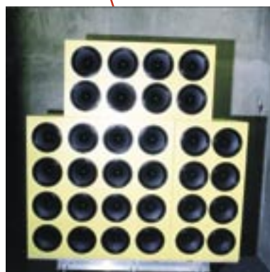
The loudspeaker room (1) contains a loudspeaker wall (10) with 32 loudspeaker units, generating wide-spectrum “pink noise” so that the sound pressure in the loudspeaker room is 110 dB(A).
