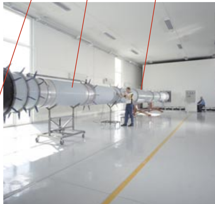
The loudspeaker room (1) and reverberation room (4) are connected by a 21-metre long measuring duct (2), in which test objects (3) are placed. The dimensions of the measuring duct can be adapted to suit the test objects concerned (both circular and rectangular).
