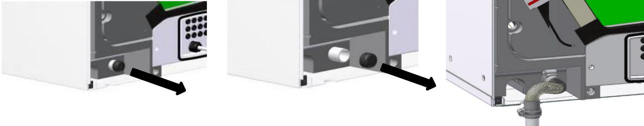
Fit a 'U' bend condensate drain having a minimum of a 60mm water seal or a HepVo valve to the building's foul water drainage system and ensure there is a minimum 3 degree fall to allow condensate drainage.
