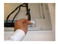
Figure 10: Insert cable opposite direction
