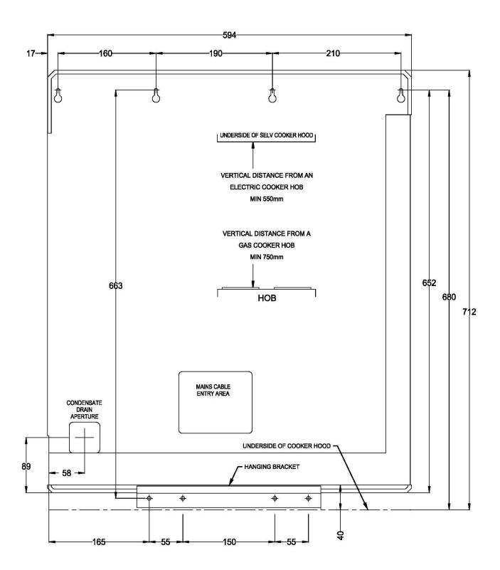
Figure 4: Sentinel Kinetic with LEFT HAND Cooker Hood Dimensions
