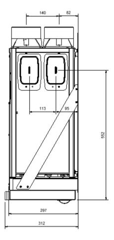
Figure 2: Sentinel Kinetic with Cooker Hood Dimensions
