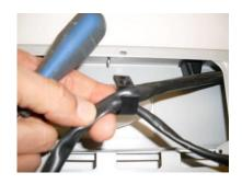
Figure 11: Using cable clip to secure the cable
