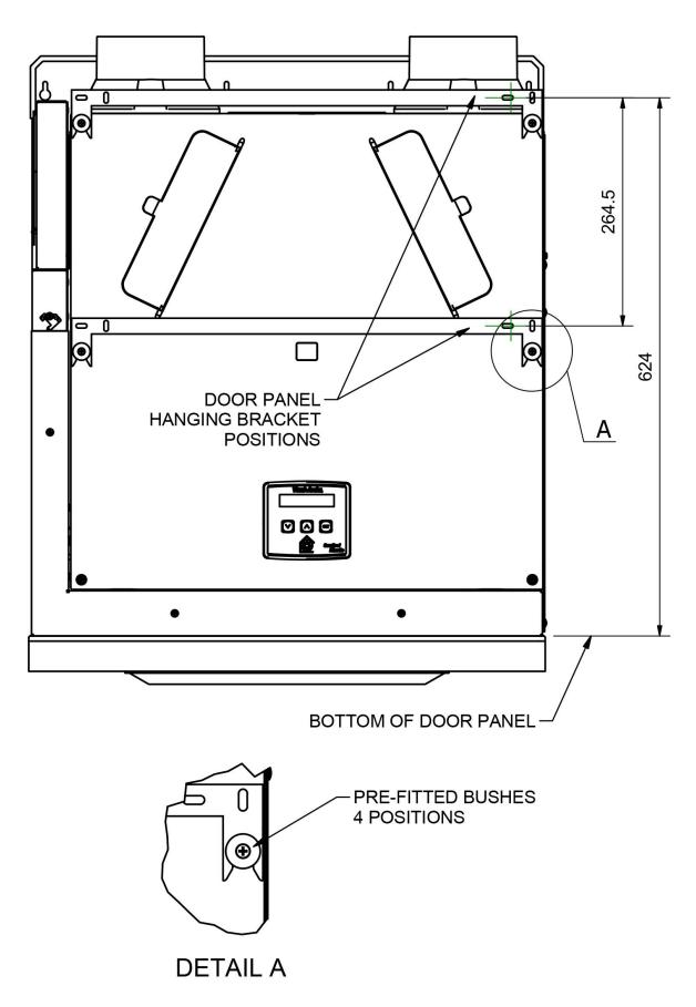
Figure 8: Door Panel Hanging Bracket Positions
