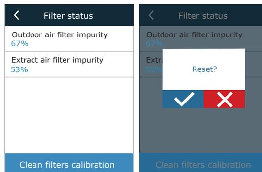
When replacing filters with filters from different manufacturers or different filtration class, calibration of clean filters is recommended. During calibration, the unit will operate at a maximum speed for a few minutes, measure the pressure difference upstream and downstream the filter and automatically determine the filtration class.
