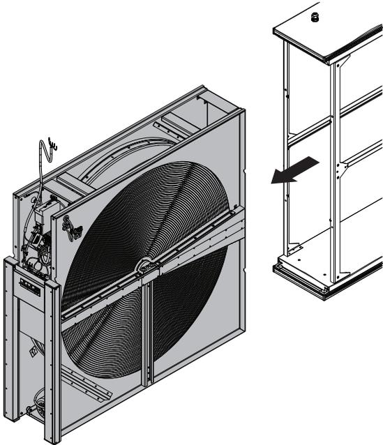
Pull the rotor completely out of the section.
