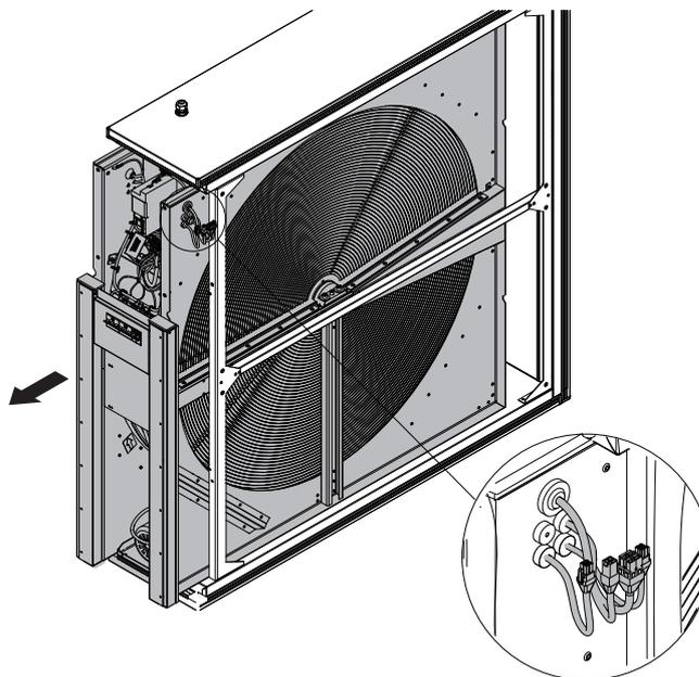
Disconnect cable connections from the filters, inspection or recirculation section side. Pull the rotor housing out of the section about 10cm. Pull the cable connections through the gap between the rotor housing and the fan section and disconnect them.
