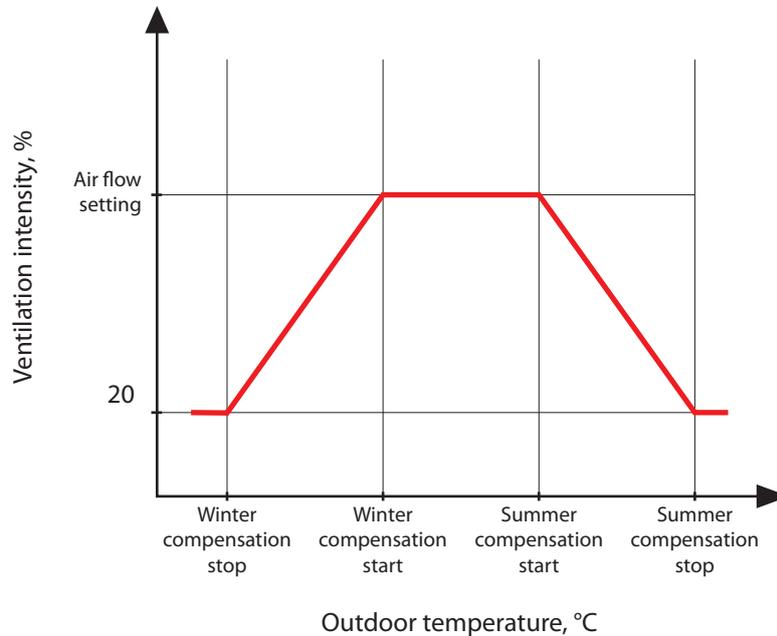
Fig. 2. OCV function operation
