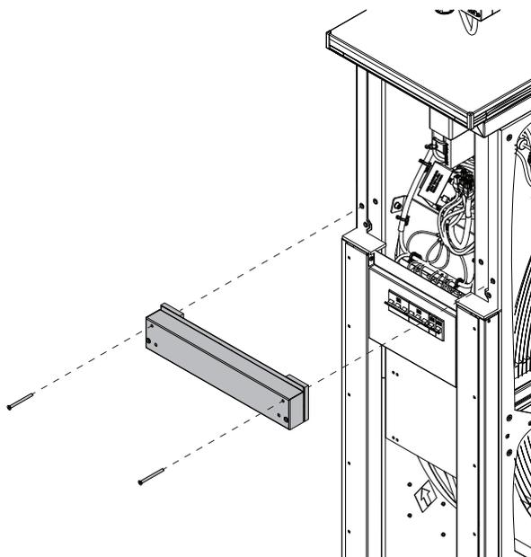
Loosen screws (2 pcs.) and remove the crossbar.
