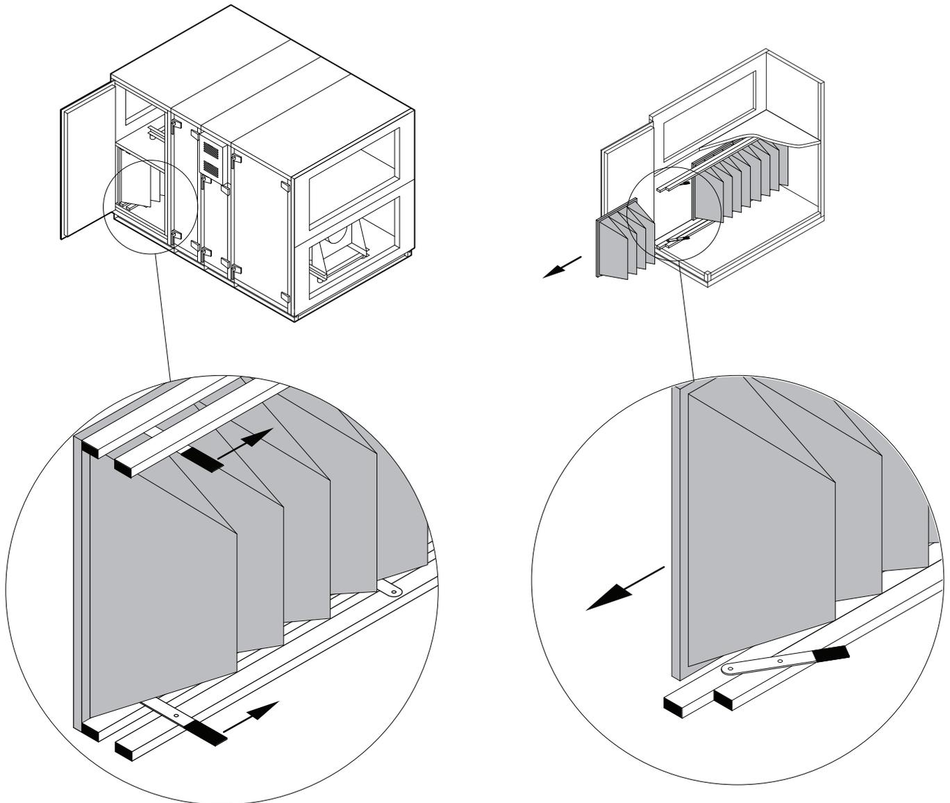
**Fig. 4.** Filter clamping device
