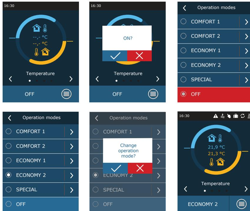
During the first minute of starting the unit, the unit automation checks the settings, automation components and opens air dampers. Later, a signal is released to fans and a heat exchanger, and the unit starts operating at a selected ventilation mode.
