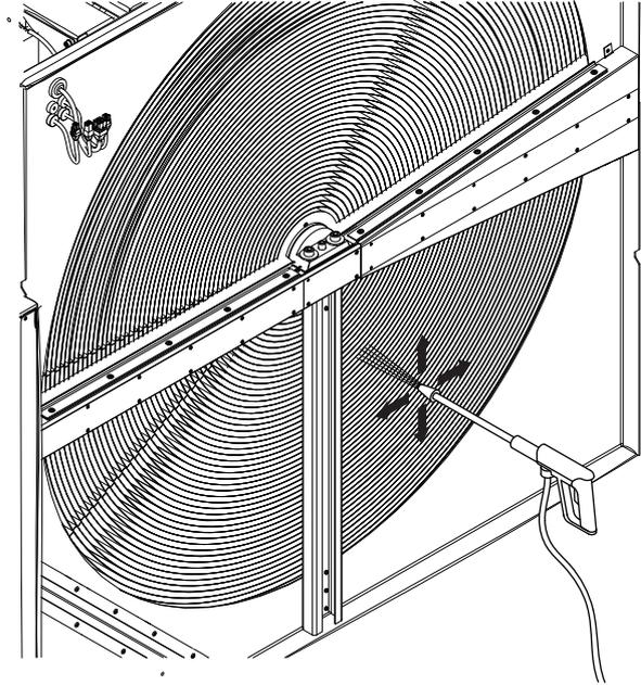
Rotary heat exchangers shall be cleaned with high-pressure washers (pressure up to 10bar). Before washing, the rotor motor and electronics must be additionally protected against moisture or dismantled. Neutral or mild alkaline detergents and disinfection agents must be used for washing. Washing agents may be harmless to the environment, shall not damage aluminium foil and shall be intended for use with high-pressure washers.
