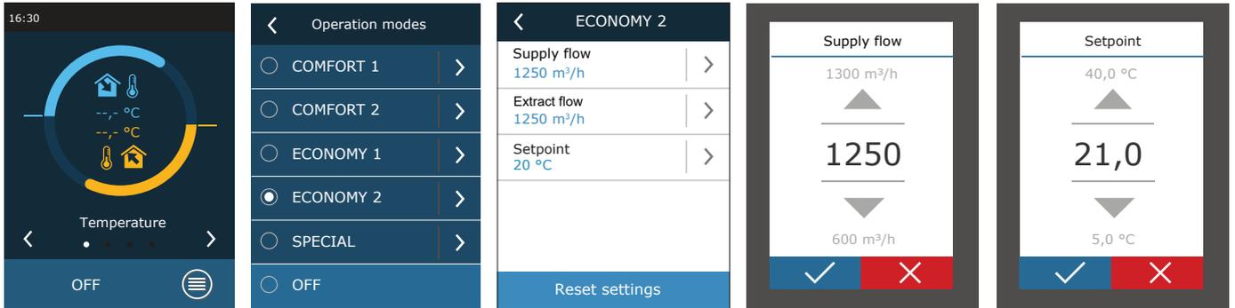
SPECIAL ventilation mode may also be used to disable heating/cooling and other functions. This saves energy when temperature and other ventilation parameters are less important (for example, at night, when the building is empty, when cooling devices can be turned off and will not be activated even when temperature exceeds the desired temperature during the day).
