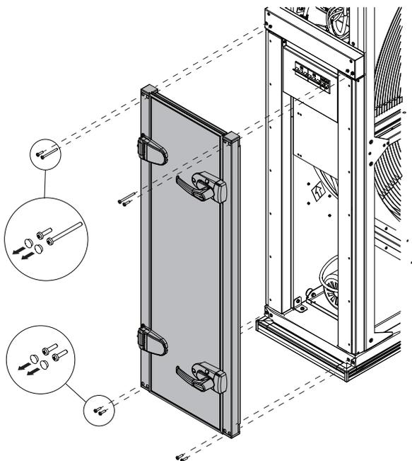
Loosen the screws holding the door struts (8 pcs.) and remove them together with the door.
