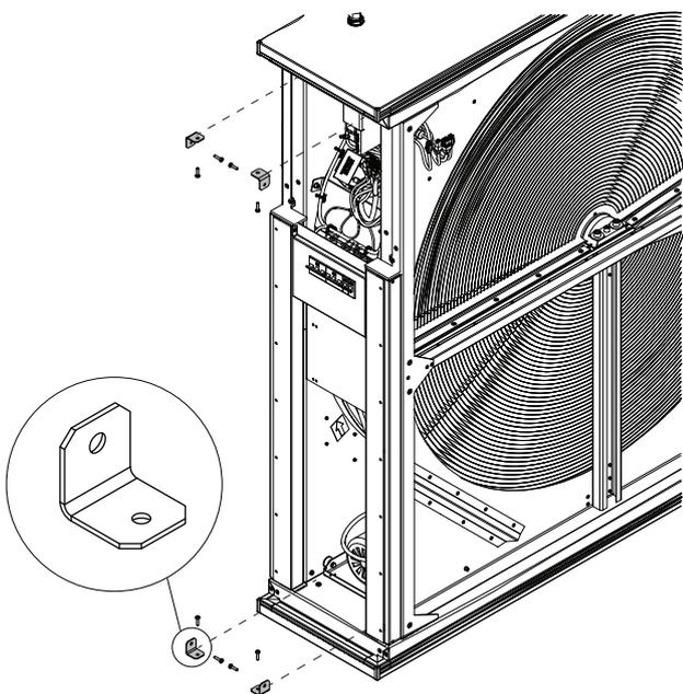
Unscrew the brackets at the corners that secure the rotor housing to the top and bottom of the section (brackets may not be used in smaller units).
