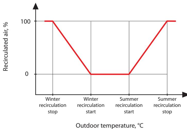
**Fig. 3.** REC function operation
